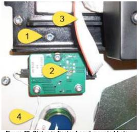
Figure 59, Status indicator board mounted below the touch screen Display module
