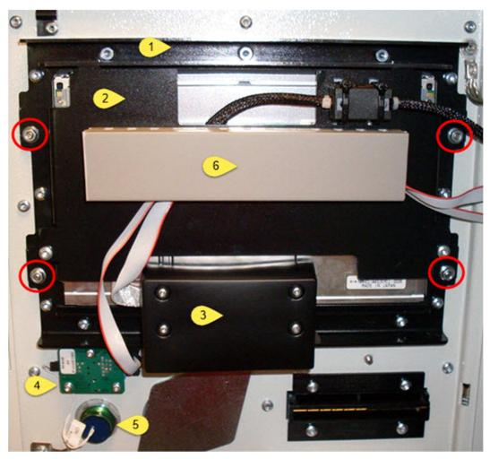
Remove the cables from the cable gutter (6)
