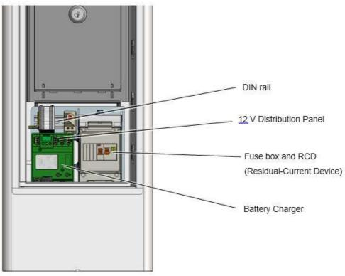
Figure 29, Pedestal interior (example)
