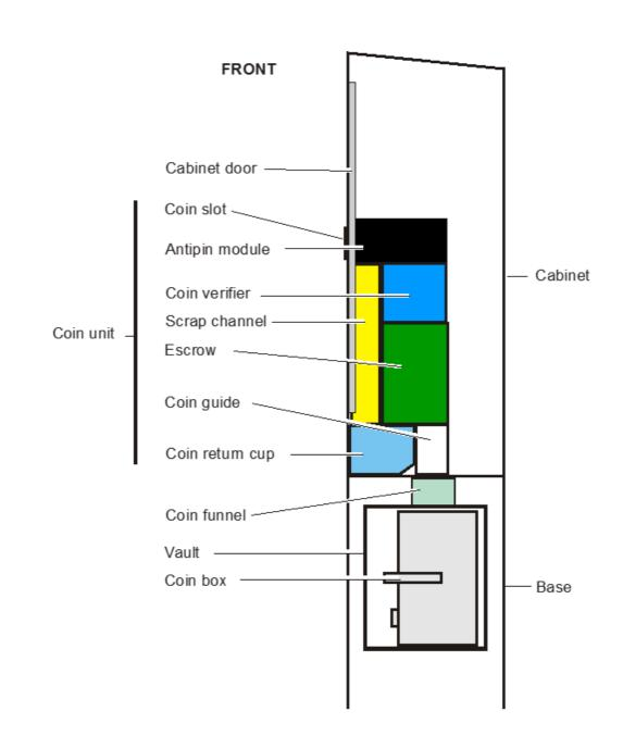
The coin unit is designed as a module that is fitted at the back of the cabinet door by means of two key holes. The module is secured with two screws that only need to be loosened slightly when the module is to be removed.
