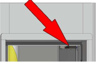
Figure 36, Door-open sensor in the cabinet.
