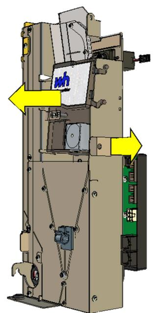
Figure 58, Removing the coin verifier Assembly
