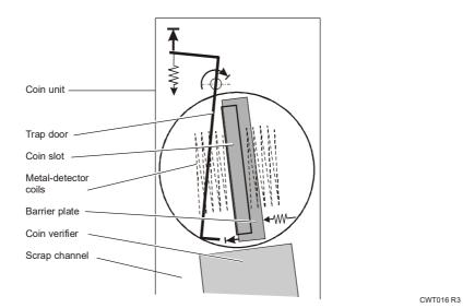
Figure 4, Anti pin in idle mode. The barrier plate covers the coin slot opening and the trap door rests in open position.
