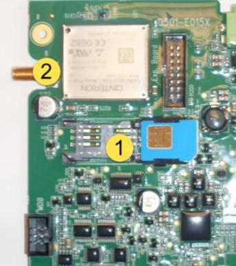
Figure 48, SIM card holder in opened position
