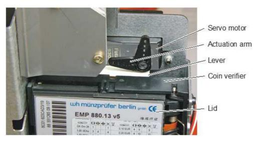
Figure 9, Coin verifier lid opening mechanism in closed position.
