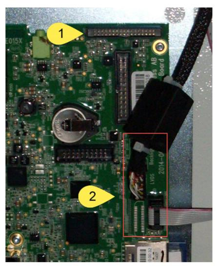
The display must be connected to the CPU board in different locations depending on the type of the display.
