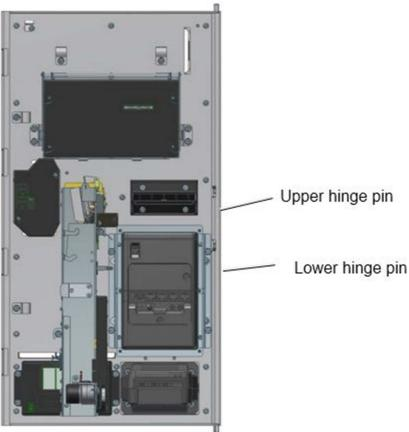
Figure 60, The door hinge mechanism.
