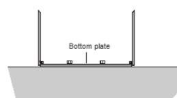
Figure 43, Terminal placed directly on the foundation
