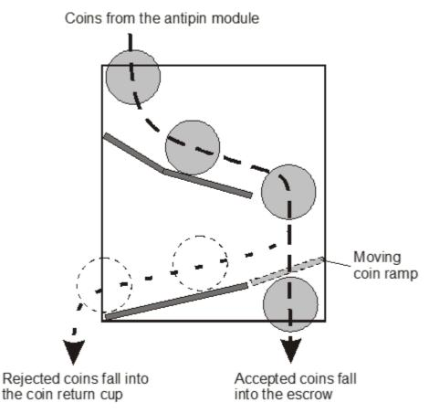
Figure 8, Coin verifier checks that a coin is valid and determines its type.
