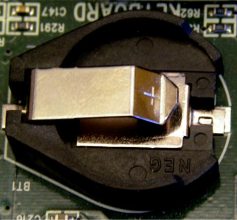
Figure 1, Backup Battery case
