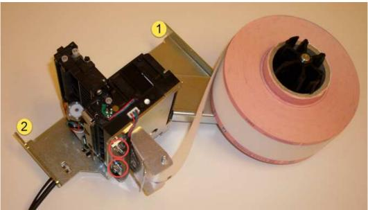
Figure 22, printer mounting on Printer shelf version 2
