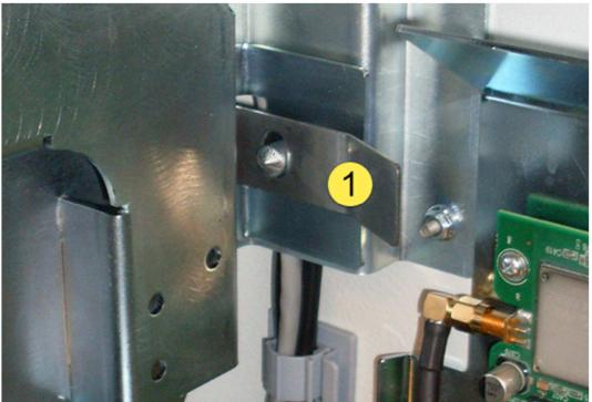
Figure 21, locking latch on version 1
