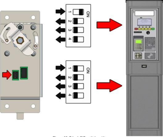
Figure 35, E-lock DIP switch settings
