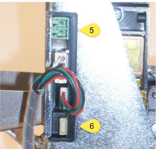
Figure 19, Power and Data connectors.
