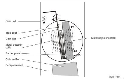
Figure 5, Barrier plate, and thus the antipin module, opens for metal objects.
