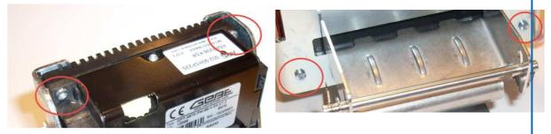
Figure 53, Mounting screws on printer shelf version 1
