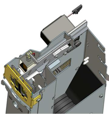
Figure 3, Anti pin module in closed position.
