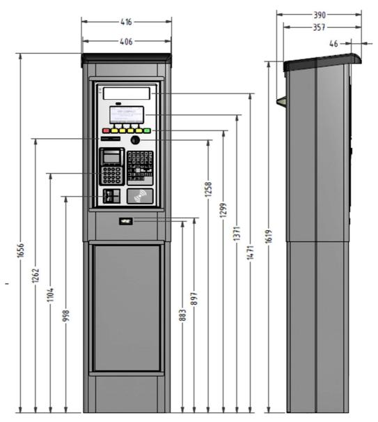
Figure 40, Terminal measurements with Xenteo
