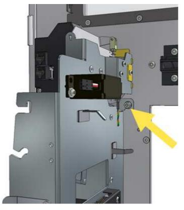
Install in reverse order. Keep the assembly pressed down while tightening the screws.
