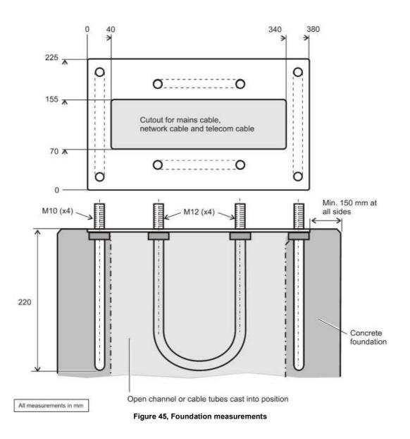
If the terminal should be connected to the grid power supply, a duct must be cast in the concrete foundation so that the cable can be routed in through the bottom of the pedestal. You can cast an approved type of plastic or steel pipe, according to local regulations.
