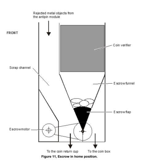
The figure above shows the coin unit as seen from the terminal's right side.
