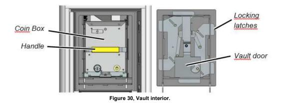
The coin box vault is made of 4 mm sheet metal with side drilling protection.
