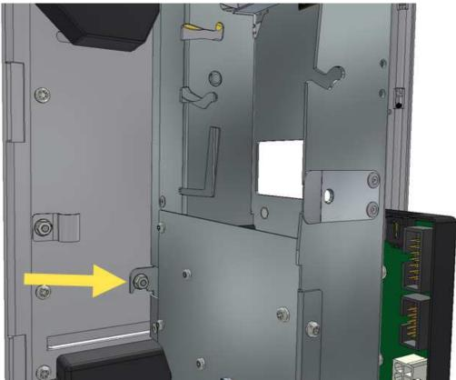
Figure 57, Removing the coin unit Assembly
