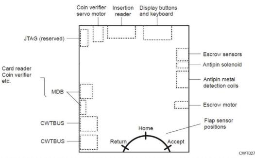
Figure 14, Coin handling board as seen from the solder side.
