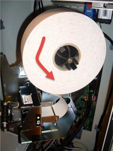
Figure 51, Paper roll mounted on a version 2 printer shelf
