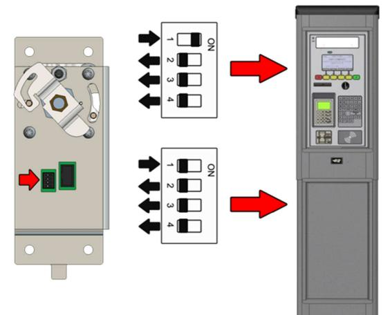
Figure 62, E-lock DIP switch settings
