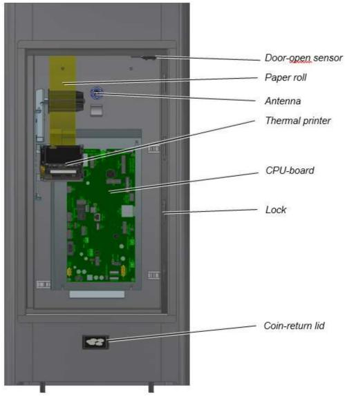
Figure 28, Cabinet interior with CPU board 0501-E0150 and GEBe printer. The printer is mounted on the version 2 printer shelf
