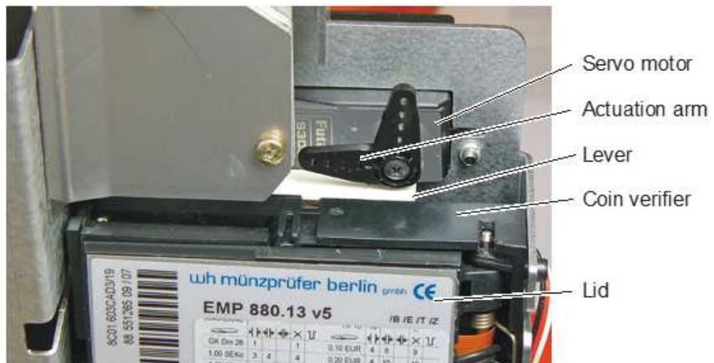
Figure 9, Coin verifier lid opening mechanism in closed position.
