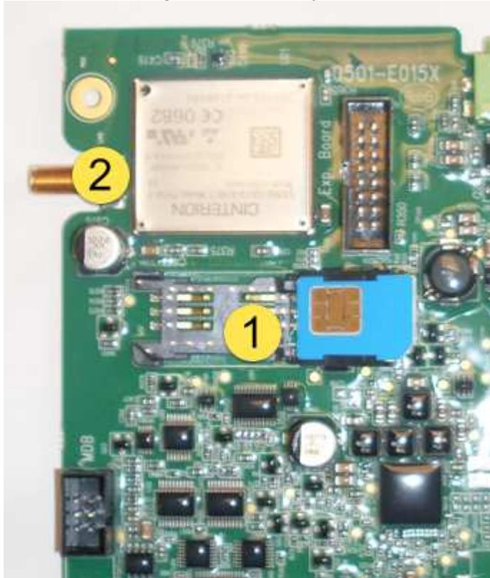
Figure 48, SIM card holder in opened position
