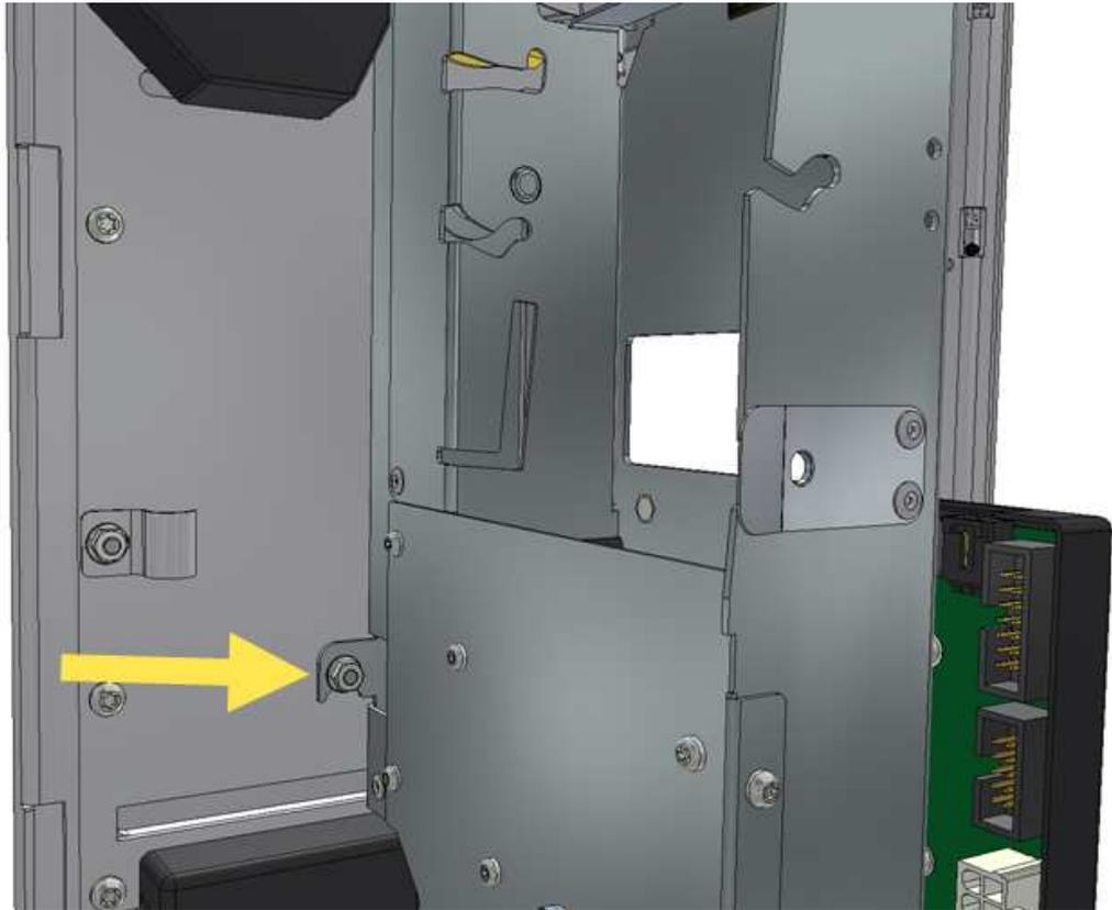
Figure 57, Removing the coin unit Assembly
