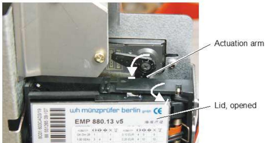
Figure 10, Coin verifier lid opening mechanism in open position.
