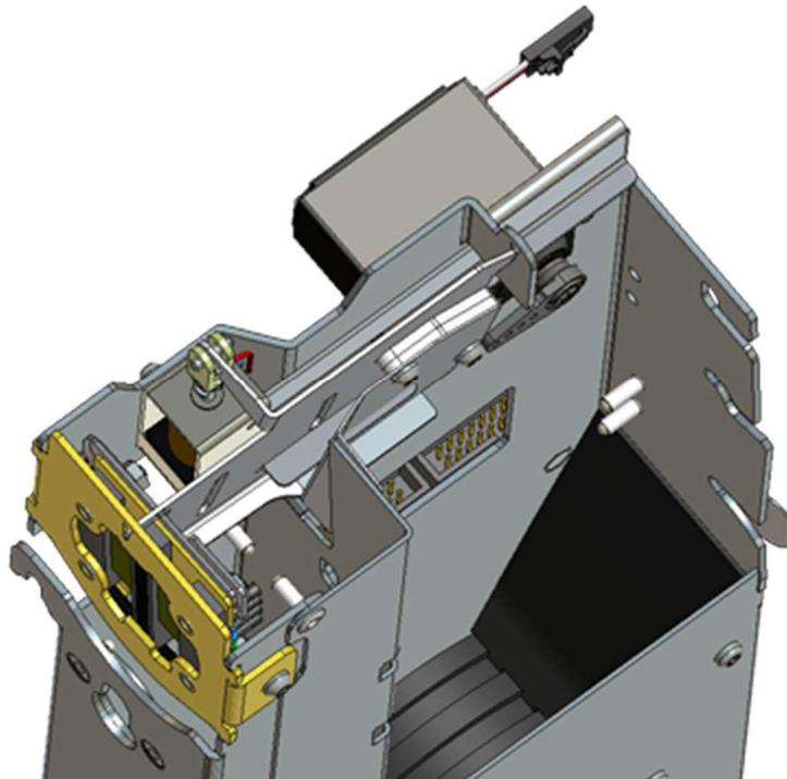
Figure 3, Anti pin module in closed position.
