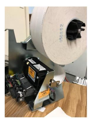
Once the paper has fed through the printer a little, you will want to push the button underneath the green light on the side of the printer to continue feeding the paper through and calibrate the printer.
