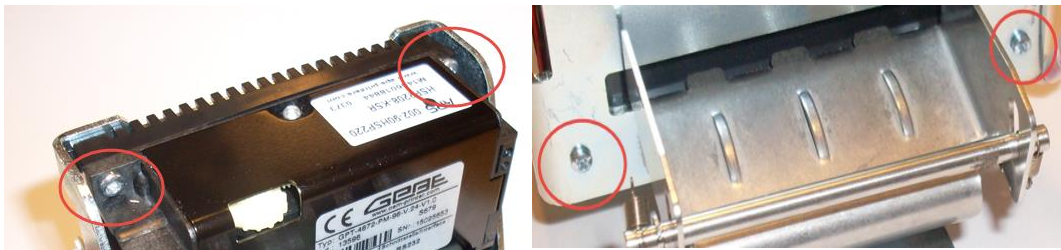
Mounting screws on printer shelf version 1
