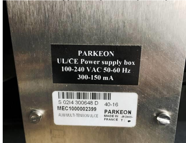
Photo 6- Power Supply Label
