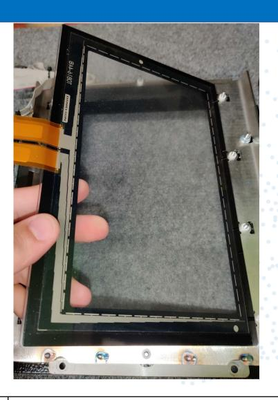
9. Place digitizer back on frame on top of the foam gasket.
