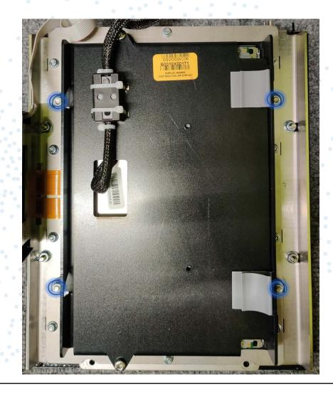
15. Install the four T10 screws into the digitizer controller board cove.
