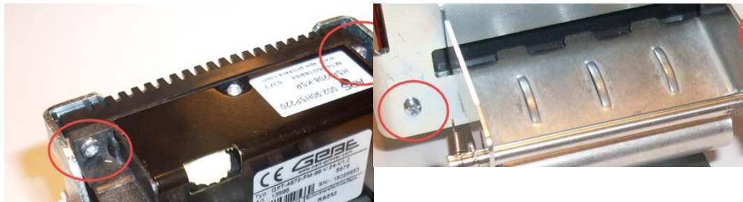
Figure 42, Mounting screws on printer shelf version 1
