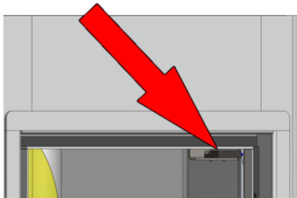
Figure 29, Door-open sensor in the cabinet.
