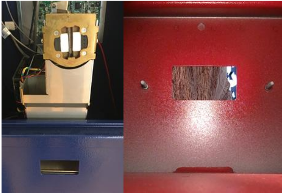
Figure 21, Coin unit with mounting bolts and Coin Return opening
