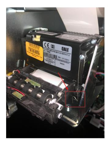
You will then want to lower the printhead by pushing down on the front and the printhead should lower.
