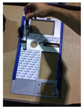
**Step 4:** The keypads are glued down with 3M double sided tape, so they would have to be removed with an object that will be able to separate it from the frame, such has a flat head screw driver or a small putty knife.
