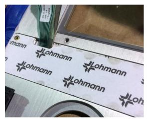
**Step 6:** Place the new keypad into the gap and press against the door firmly so the tape contacts the door.
