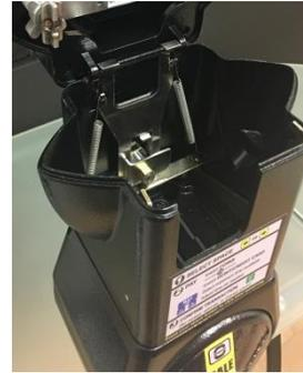
1. Attach battery to grey cover using existing Velcro and connect battery plug. (Be sure to clip cover back into Mechanism)
