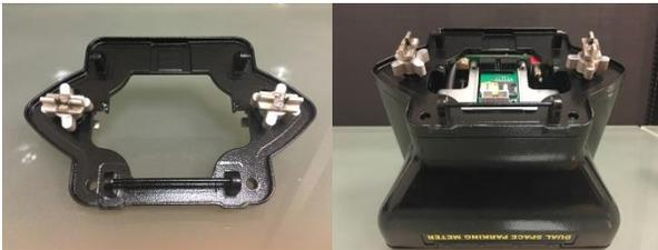
4. Attach complete upper unit using the hooks on lower housing and prepare coin unit.
