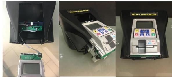
3. Mount middle bracket to bottom of upper housing and tighten the fixed silver screws.
