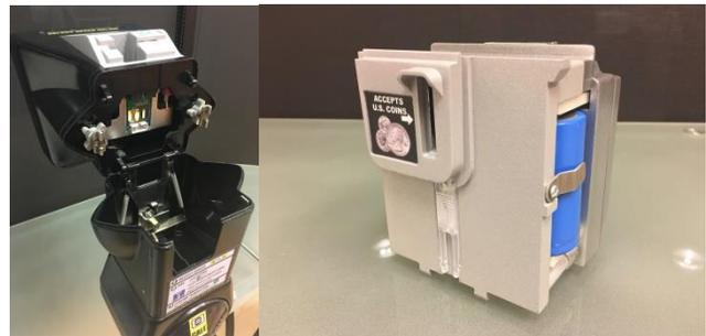
5. Place coin unit into lower housing and connect ribbon cable.
