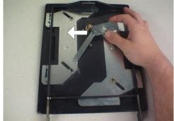
19. Push the lever assembly arm down onto the lock. Make sure that the lever assembly is flush with the lock. Also make sure that the metal tab on the lock is not underneath the metal plate.
