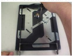
18. Pull up and swing the lever assembly arm back over the lock.
