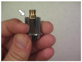
14. Insert the lock into the vault door. Make sure that the metal tab is on the **right** side of the lock.
