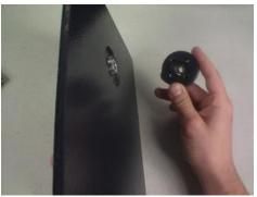
11. Push on the lock, which will remove it and the bezel from the vault.
