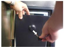
4. Remove the vault from the vault frame. Do this by pushing the bottom of the door up; then pull the door away from the frame.
