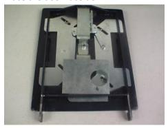
6. Remove the 10mm nut and the metal bar that the 10mm nut secures down.
