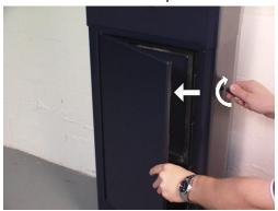
2. Now insert the vault door key into the coin vault door, turn the key clockwise and use your hand to gently drop the coin vault door until it is in a stable position.
