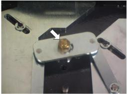
21. Take the metal bar and slide the one end into position, then lower it into place. The stud on the vault door should insert into the hole on metal bar.
