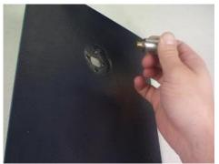
12. Now that the old lock has been removed, a new lock can be installed. Start by orienting the vault door so that the hinge hooks are at the bottom.
