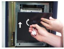
24. Shut the vault door and lock it by turning the key counter-clockwise.
