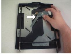
9. Unscrew the two screws that are located to the left and right of the lock.
