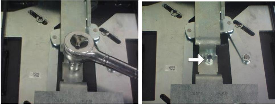
22. Reinstall the vault door back onto the vault frame.
