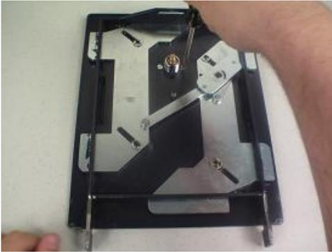
18. Pull up and swing the lever assembly arm back over the lock.
