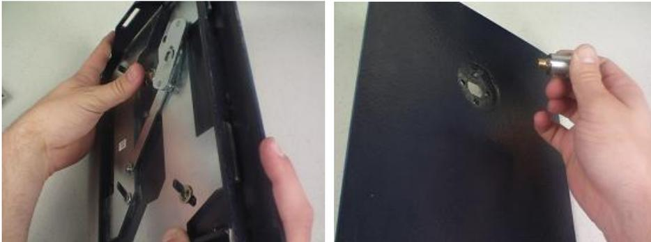
12. Now that the old lock has been removed, a new lock can be installed. Start by orienting the vault door so that the hinge hooks are at the bottom.
