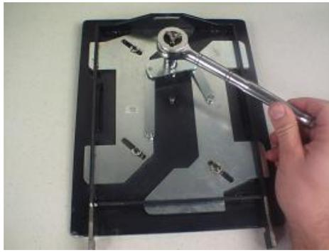
8. Lift up on the lever assembly arm and move it to the right.
