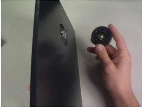
11. Push on the lock, which will remove it and the bezel from the vault.
