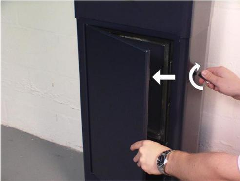
2. Now insert the vault door key into the coin vault door, turn the key clockwise and use your hand to gently drop the coin vault door until it is in a stable position.
