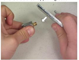
16. Now that the old lock has been removed, a new lock can be installed. Start by orienting the lock assembly so that the gear arm is to the **Right** of the center hole.
