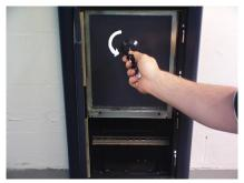
36. Finally, shut and lock the bottom door.
