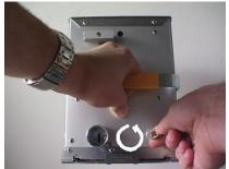
34. Once the coin box has been reset; place the coin canister in the coin vault.
