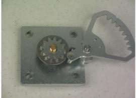
21. Without spinning the bottom washer and the gear, carefully press on the lock and pull up on the washer and gear. This will allow for the gear arm to swing into place.
