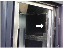
6. Remove the three 10mm nuts that are accessible. It will be easier if the socket wrench has an extension on it.
