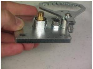
19. Now take the washer with the arch cut-out on it and place it on top of the lock assembly. Make sure that the metal tab is visible in the arch cut-out. You do not want to have the metal tab underneath the washer. Also make sure that the cut-out is horizontal. (Refer to the picture for orientation.)
