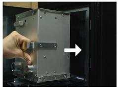
35. With the key turned to the right as far as possible. Gently raise up the vault door until it is flush with the vault cage. Now lock the vault door by turning the key counter-clockwise and removing it.
