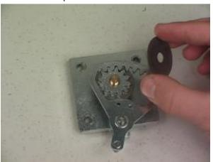
13. Push on the Lock so that the gear arm can move freely; then swing the gear arm away from the lock.
