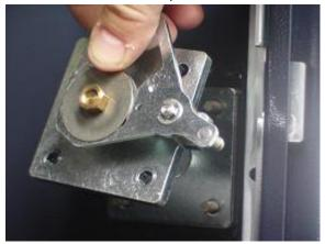
11. Now that the Assembly has been removed, remove the 11mm nut.
