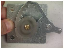
25. Install and tighten down the 11mm Nut. Do Not torque down the 11mm nut, doing so will cause the lock not to spin.
