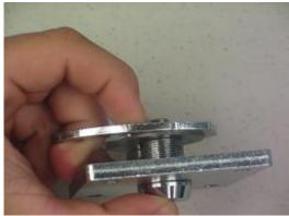
24. Now place the top washer on top of the gear arm.
