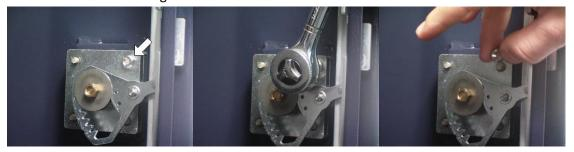
9. Turn the key counter-clockwise; then remove the Key.
