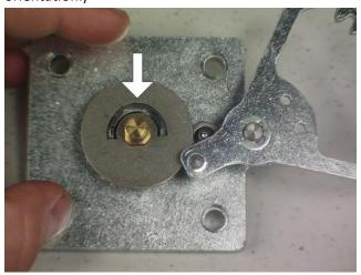
20. Take the gear and line up the inner square center with the square section on the lock. Place the gear on the lock on spin it until the gear is flush with the bottom washer.
