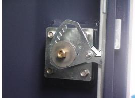
28. Once the lock assembly is installed correctly; tighten down the three 10mm nuts that are accessible.
