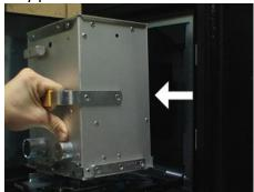
5. Locate the lock assembly behind the coin vault frame. It is positioned inside the cabinet on the opposite side of the key hole.
