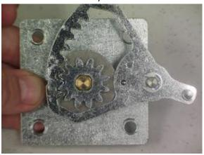
23. Now press on the lock to make the gear become flush with the gear arm. Also make sure the bottom washer is flush with the bottom of the lock. If the washer or the gear spins and does not become flush; then remove the gear and washer and star back on step 17.
