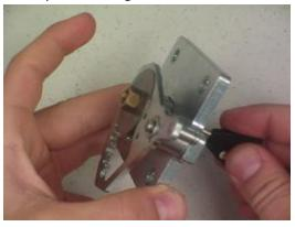
27. Now install the lock assembly back into the meter. Make sure the stud on the lock assembly is inserted into the hole on the locking bar. You may have to lift up on the locking bar for the stud to be installed correctly.
