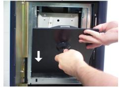
4. Turn the latch lever on the front of the coin box in a clockwise direction, making the latch lever horizontal, and then carefully pull the coin box out.
