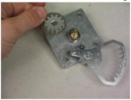
15. Remove the old lock by pushing it out.
