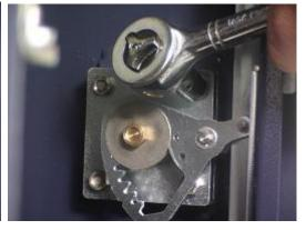
31. Once the lock assembly is secured; turn the key a few times to test the functionality of the lock.
