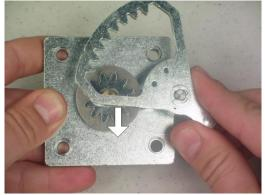
22. Make sure that gear is all the way to the bottom of gear arm as possible. (Refer the picture for the correct orientation.)
