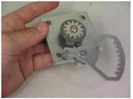
14. Now remove the bottom washer and the gear.
