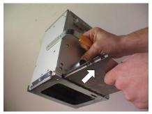
33. Close the bottom of the coin box. Now turn the key to the left, which will lock the box and allow for the box to be placed into the meter.
