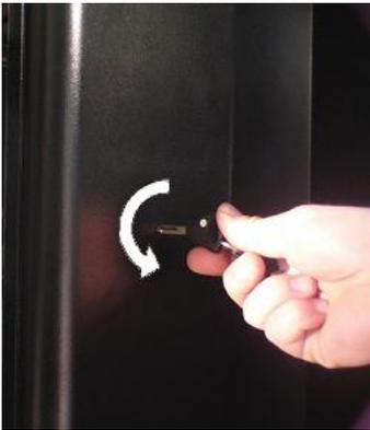
3. Insert your key into the coin vault door, turn the key clockwise and use your other hand to gently drop the coin vault door until it is in its stable position.
