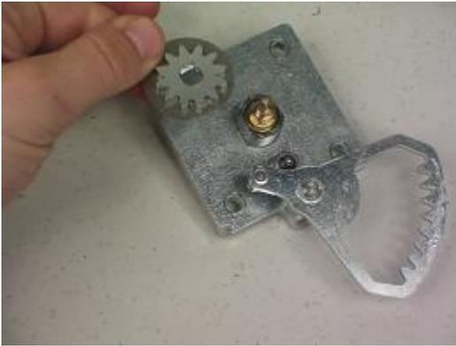
15. Remove the old lock by pushing it out.
