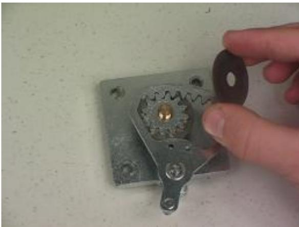
13. Push on the Lock so that the gear arm can move freely; then swing the gear arm away from the lock.
