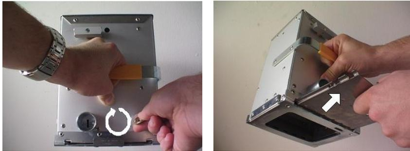
33. Close the bottom of the coin box. Now turn the key to the left, which will lock the box and allow for the box to be placed into the meter.
