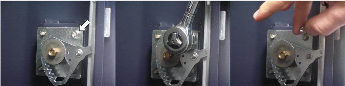
9. Turn the key counter-clockwise; **then remove the Key.**
