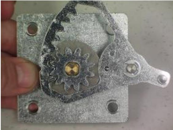
23. Now press on the lock to make the gear become flush with the gear arm. Also make sure the bottom washer is flush with the bottom of the lock. If the washer or the gear spins and does not become flush; then remove the gear and washer and star back on step 17.
