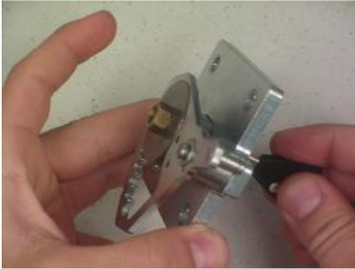
27. Now install the lock assembly back into the meter. Make sure the stud on the lock assembly is inserted into the hole on the locking bar. You may have to lift up on the locking bar for the stud to be installed correctly.
