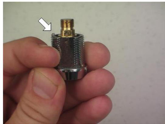
18. Insert the lock into the lock assembly. Make sure the metal tab is on the opposite side of the gear arm.
