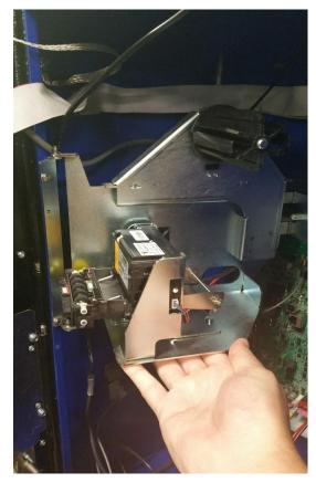
Looking at the rear of the printer, reseat all 4 cables from the right side of the printer and 1 from the left
