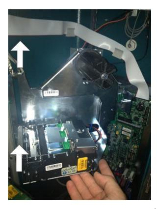
Remove all 3 cables from the back of the printer
