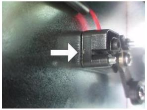
E. Install and tighten the 5.5 mm nuts to secure the collection switch in place.
