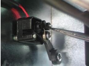
D. Make sure that the collection switch is flush with the coin box cage.
