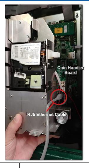
Connect the RJ5 to the coin handler board on the coin unit.
