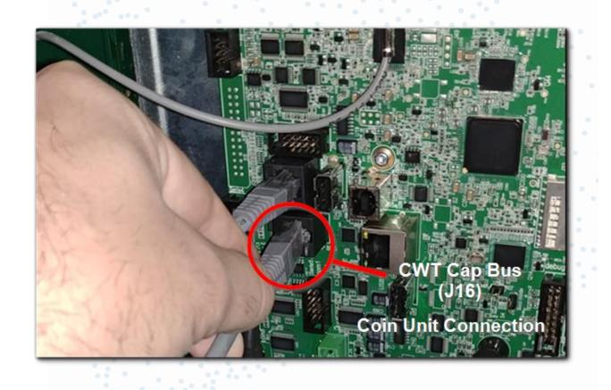
FLOWBIRD MOUNTIING THE NEW COIN UNIT MPC TO CWT STEALTH
