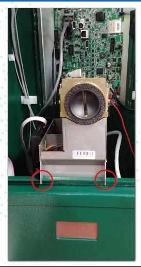
FLOWBIRD MOUNTIING THE NEW COIN UNIT MPC TO CWT STEALTH
